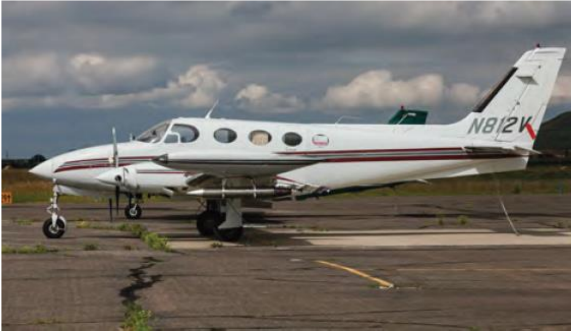
Figure 9: Cessna 340A: Used for Hail suppression operations with torches (Langerud, 2015)
